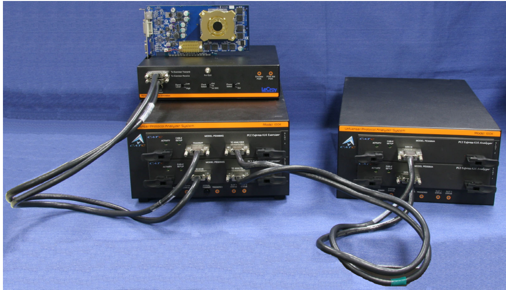
Figure 3.8 PETrainer EML (bottom left) connected to a Host Emulator adapter (top) and a PETracer EML Analyzer (right). The Host Emulator has a PCI Express graphics card inserted.
